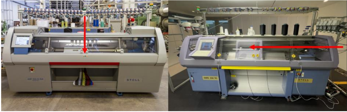
Figure 7: The examined flat knitting machines for the laboratory (left) and production-like (right) measurement campaigns with visualized feeding direction (red arrows).
