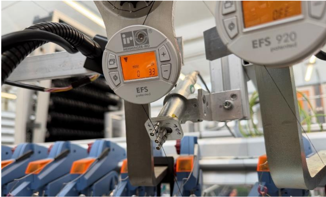
Figure 4: Modified feeder and 3-roller thread tension sensor mounted statically above the machine.
