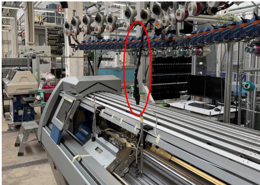
Figure 3: SE8 directional microphone (red circle) mounted above the knitting section of the machine.
