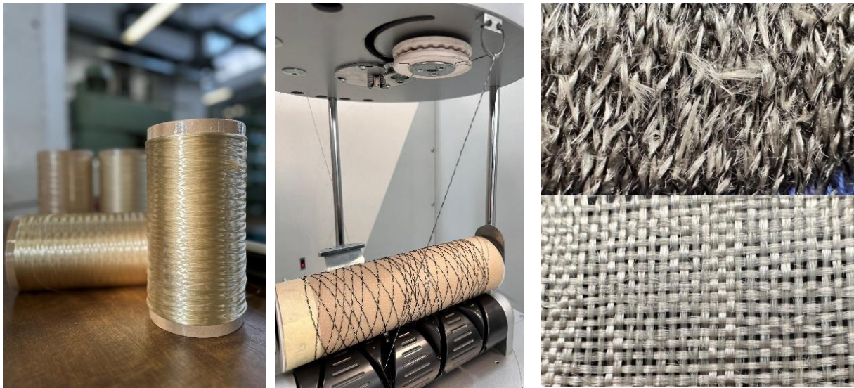
Figure 7: Chitin multifilament yarns spun from EMIMOPr (left) Twisting trials with chitin multifilament yarn on a laboratory double-yarn twisting machine (DIRECTWIST, AĞTEKS Ltd.) (middle); knitted sample with viscose support yarn (black) (top right); plain-woven fabric made from pure chitin yarn (bottom right)
