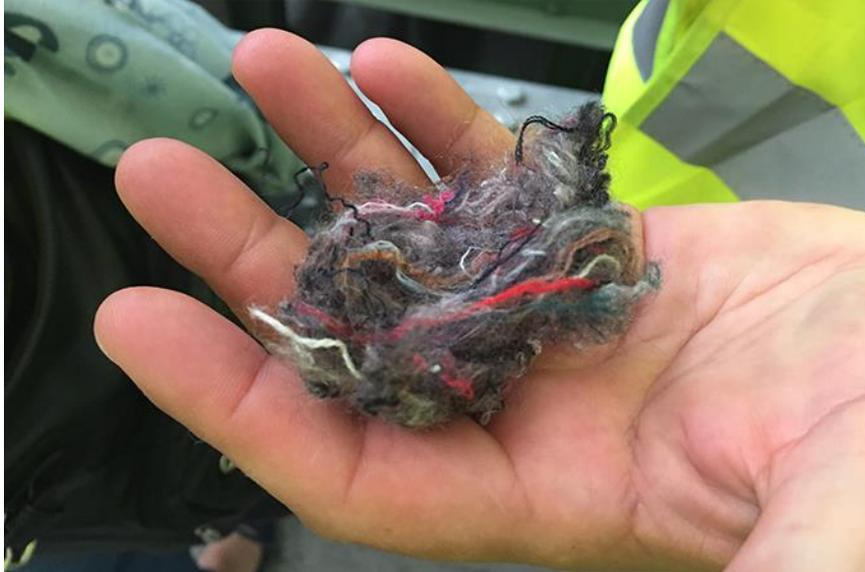
Recycled end product, which is later used to produce automotive insulation.
