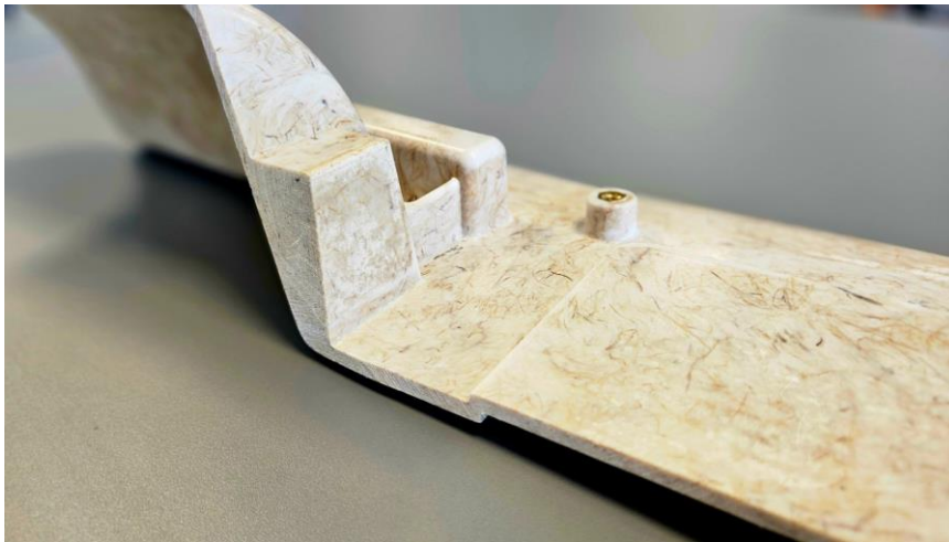
Close-up of a component made of natural fibre SMCs (train interior cladding). The geometric degrees of freedom that the material allows are clearly visible in addition to the fibre flow. Photo Fraunhofer IWU
