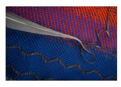
An MIT team has designed an "acoustic fabric," woven with a fiber that is designed from a "piezoelectric" material that produces an electrical signal when bent or mechanically deformed, providing a means for the fabric to convert sound vibrations into electrical signals. Credits: Image Greg Hren
