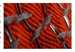
In the new work, the researchers flipped that idea to create a fabric loudspeaker that can be used to cancel out soundwaves.
