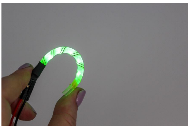
The strip's 3D structure transforms it from flexible to stretchable
