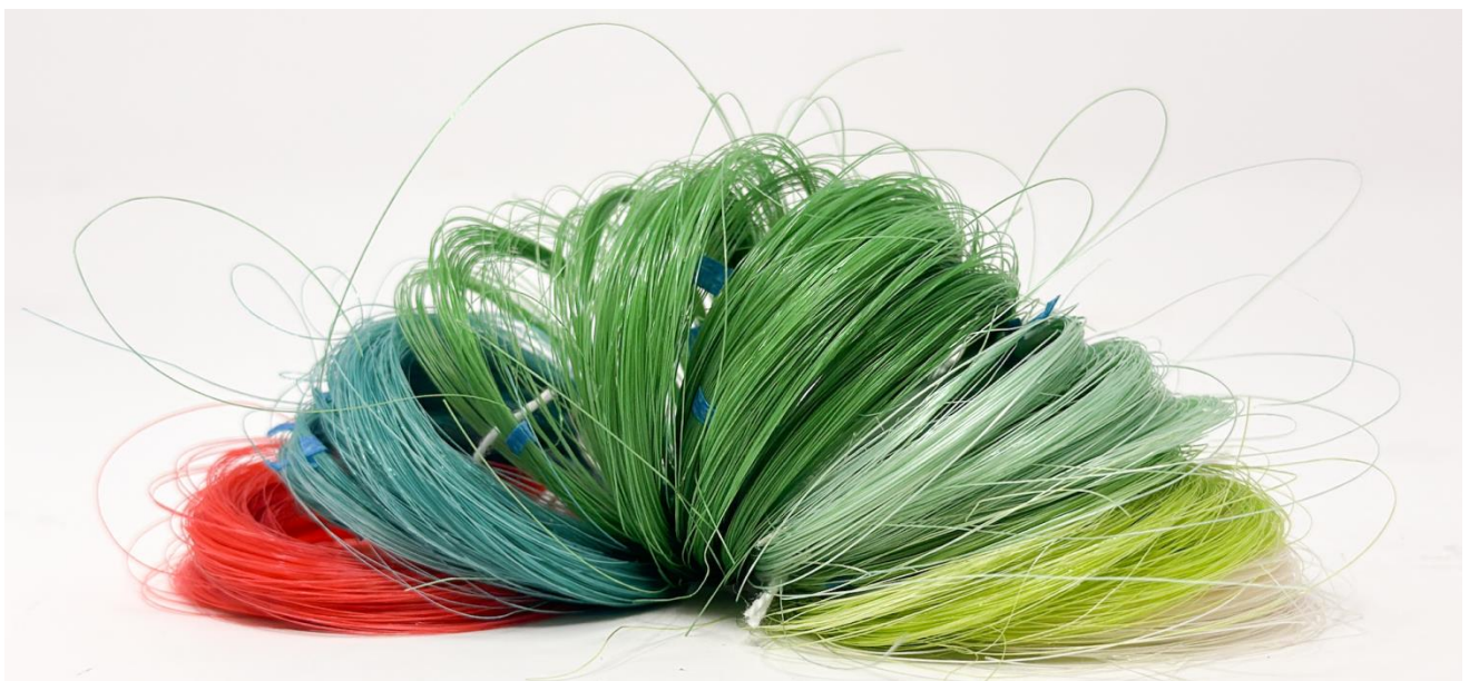
Biofibers made from gelatin in a rainbow of colors. (Credit: Utility Research Lab)
