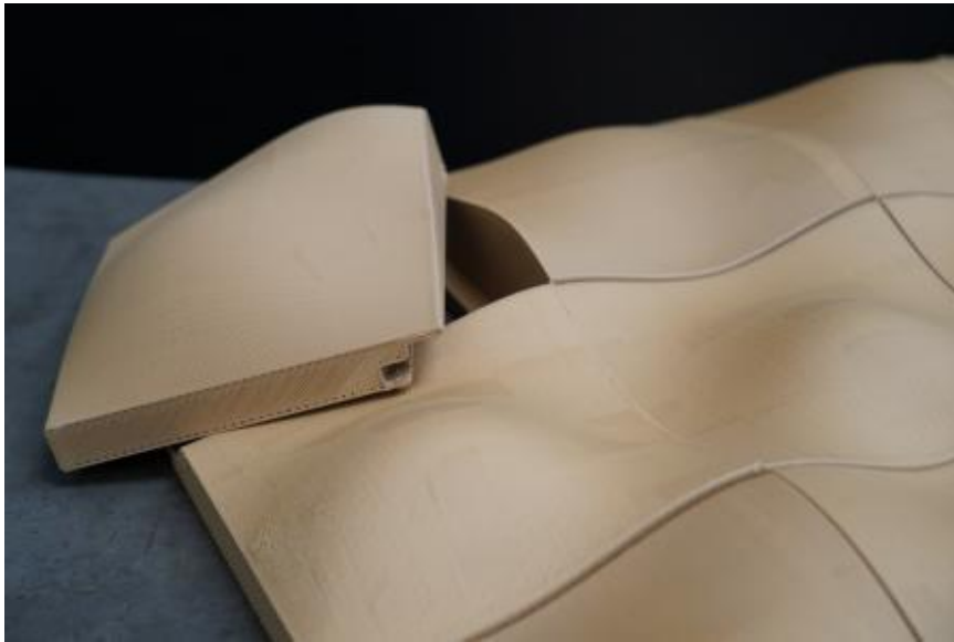
First tests with free-form tiles made of wood short fiber filament. (Photo: LZH)
