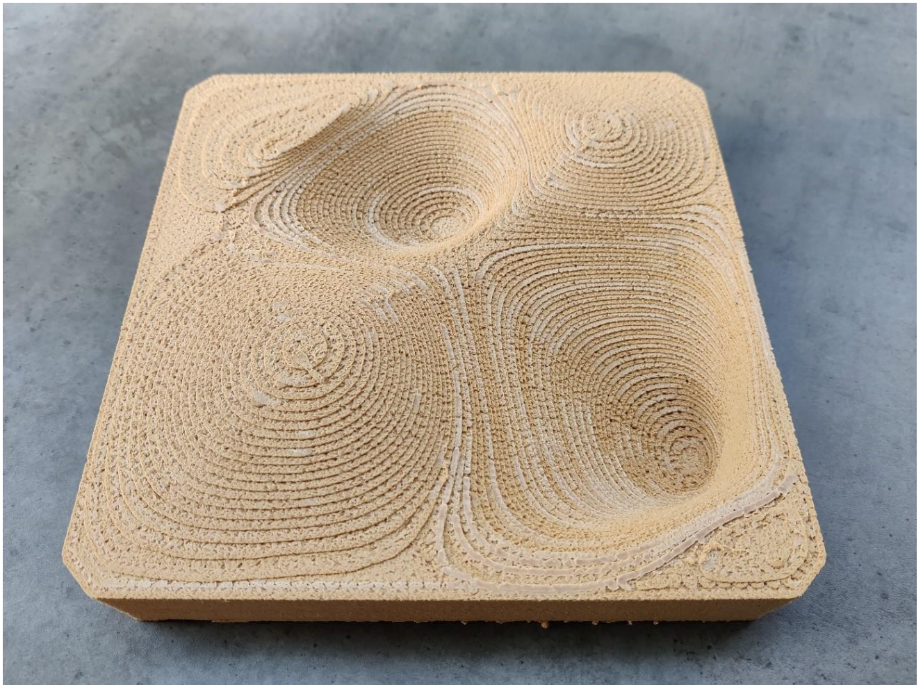
In the project 3DNaturDruck, construction elements will be manufactured additively from natural fibers, such as here a free-form tile made of wood short fiber filament (Photo: LZH Laser Zentrum Hannover e.V.).
