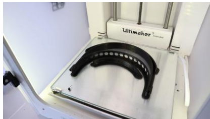
Manufacturing process: Fused Deposition Modeling (FDM)
