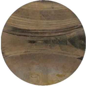
Caption: Signs of wear to the pressure disk after 24 hours of operation using the old fixing system with deactivated thrust pad rotation
