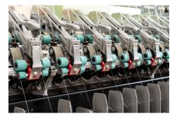
COMPACTeasy is a compacting device available as plug-on/plug-off solution.
