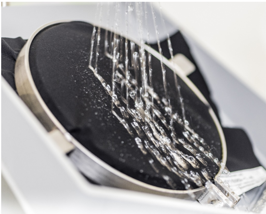
Image: Evaluating the DWR performance using the spray test method at HeiQ laboratories (HeiQ)
