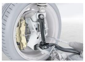
For the first time in a serial-produced car, the stabilizers on the front and rear axles are made of carbon, as well as their coupling rods – all with outstanding performance.
