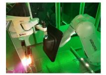
Automated fibre placement (AFP) processes produce a lot of uncured prepreg tape material scrap because all reels of tape are simultaneously changed as soon as the tape left on one reel is not enough to place the next layer of the laminate. With large AFP systems that process up to 32 reels in parallel, manufacturers suffer from high scrap rates of ~10%.
