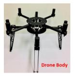
The existing CFRP (carbon fibre-reinforced plastic) drone was brittle at low temperatures and the many CFRP parts were damaged in the event of a collision, resulting in breakage.
