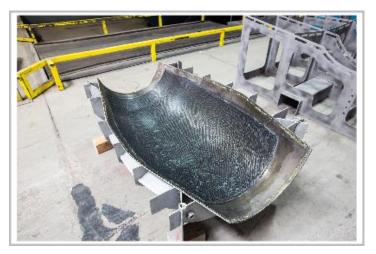
HyVarC<sup>®</sup> is a patent-pending hybrid InVar and carbon fibre composite layup mould. HyVarC<sup>®</sup> layup tooling offers a high-precision, lightweight, short lead time solution for prototype and development applications.
