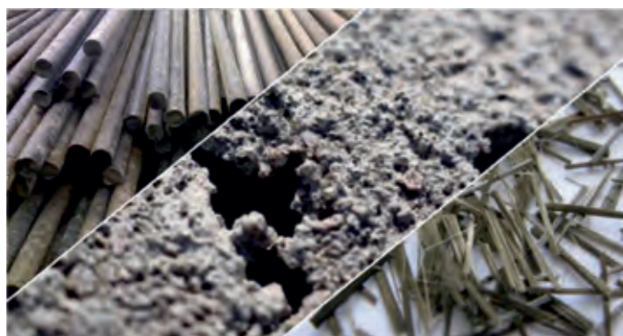
Fig. 2 Concrete made from basalt fiber
