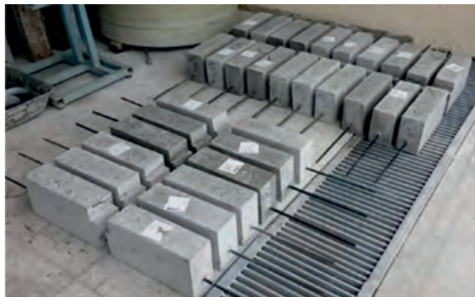
Fig. 3 Bricks made of basalt fiber
