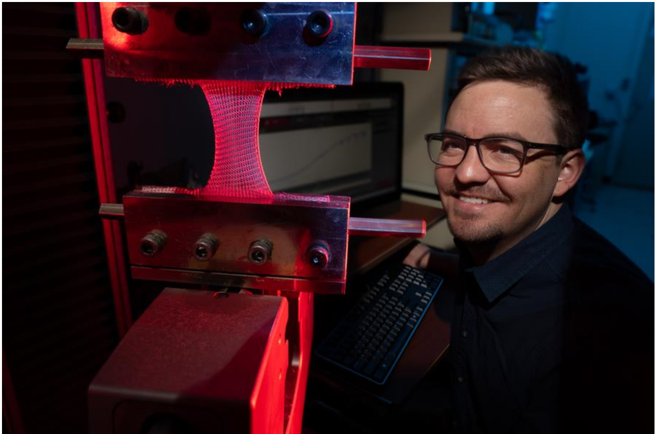
Lincoln Laboratory staff member Steve Gillmer tests the elasticity of a bioabsorbable fabric in order to compare its stiffness to different types of human tissue. Credits:Photo: Glen Cooper/Lincoln Laboratory
