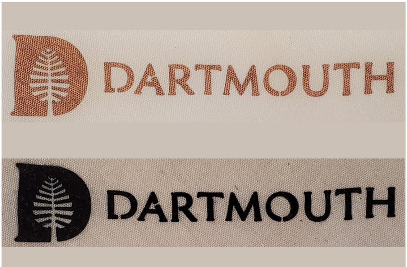
Copper imprinted on fabric (top) is replaced with a metal-organic framework (bottom) capable of detecting and capturing toxic gases. Photo: Katherine Mirica
