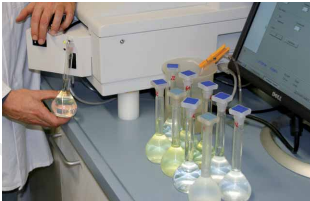
Determination of formaldehyde with a UV/VIS-spectrometer according to Japanese Law 112
